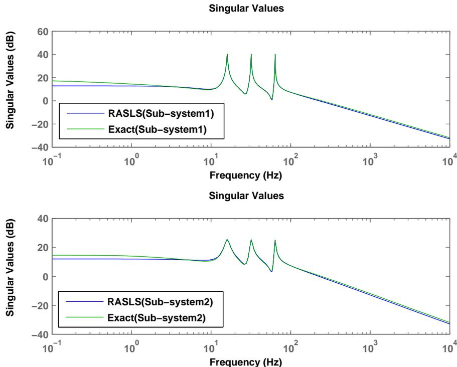
FIGURE 1. Largest singular value of the frequency response of the original system (sub-system 1) of order 1006 and reduced one of order 10 to a frequency range with RASLS method
