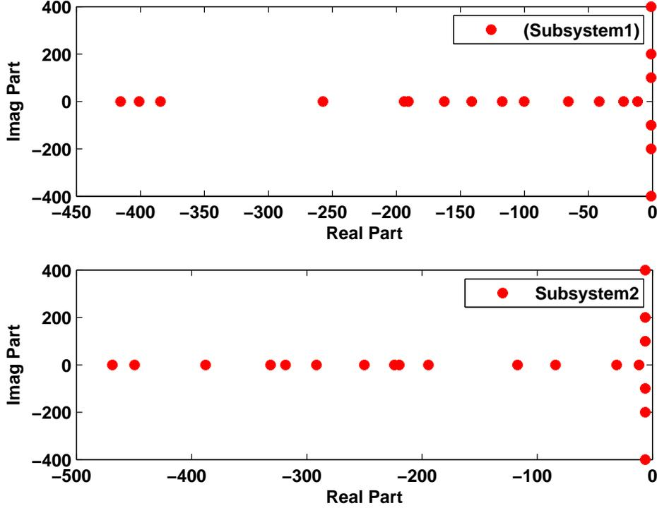
FIGURE 3. Pole Distribution of FOM reduced system (order 10) with RASLS method
