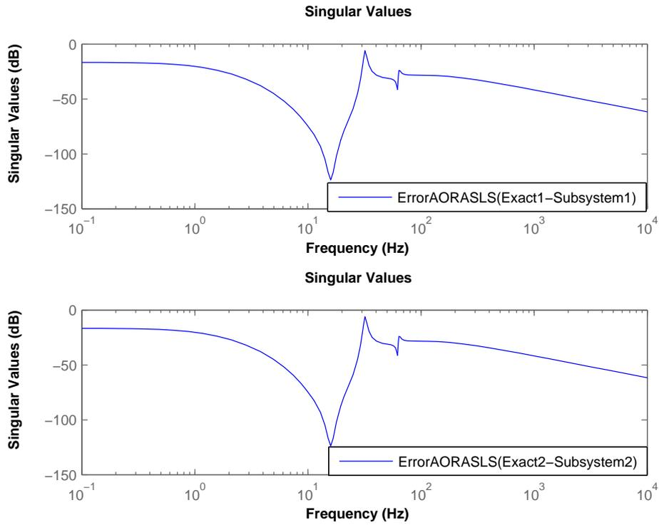
FIGURE 5. Absolute error system between original system of order (1006) and the reduced one of order (10) with AORASLS method
