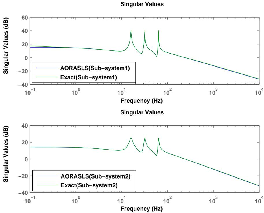
FIGURE 4. Largest singular value of the frequency response of the original system (sub-system 1) of order 1006 and reduced one of order 10 to a frequency range with AORASLS method
