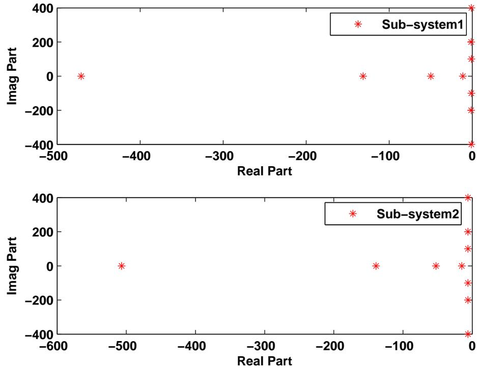
FIGURE 6. Pole Distribution of FOM reduced system (order 10) with AORASLS method
