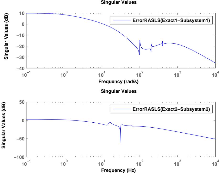
FIGURE 2. Absolute error system between original system of order (1006) and the reduced one of order (10) with RASLS method
