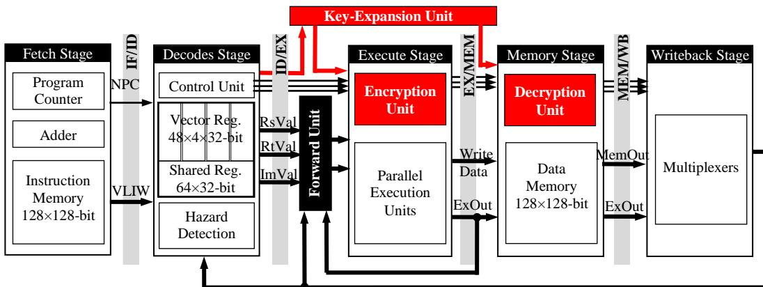
Fig. 4. Block diagram of CryptoVVSHP.
