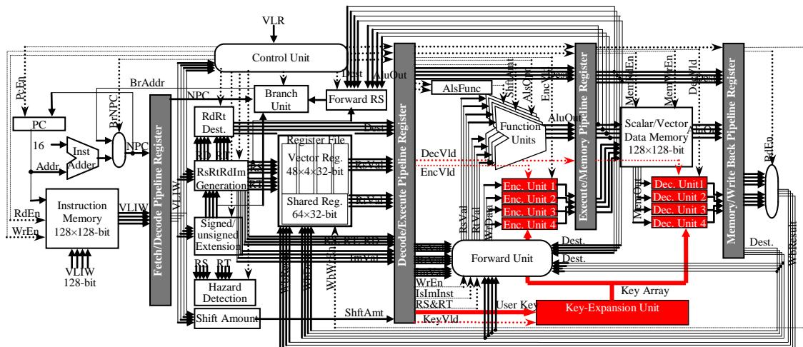
Fig. 5. CryptoVVSHP datapath for executing encrypted scalar/vector data.
