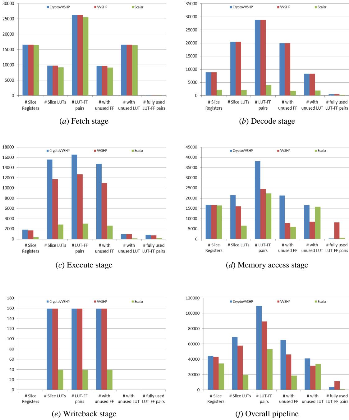
Fig. 8. Synthesizing CryptoVVSHP, VVSHP, and scalar pipelines on FPGA Virtex-5.
