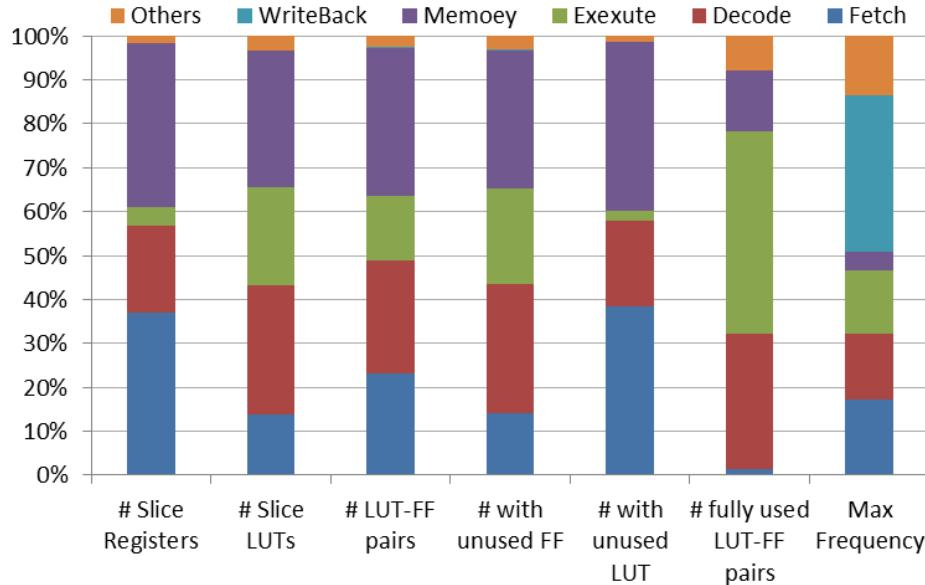
Fig. 7. Percentage of complexity in each stage of CryptoVVSHP.
