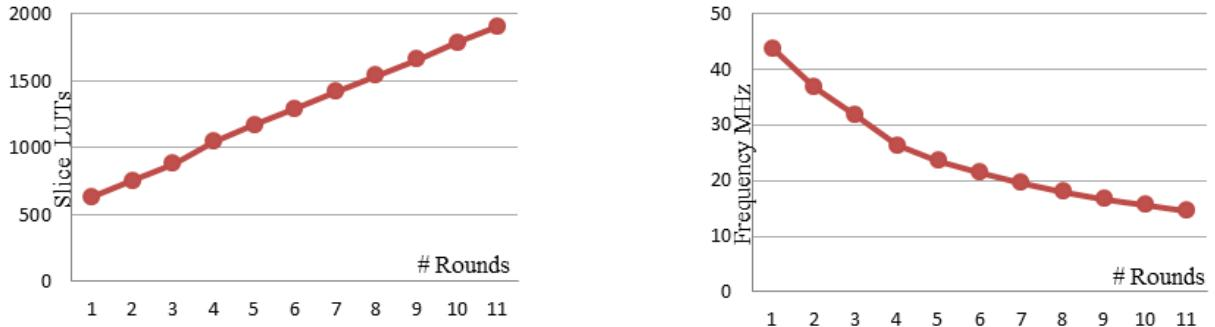
Fig. 3. FPGA implementation of decryption algorithm with  $r$  rounds.
