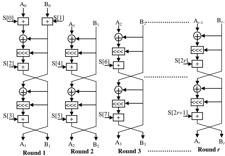
Fig. 1. Unrolled RC5 encryption algorithm with  $r$  rounds.
