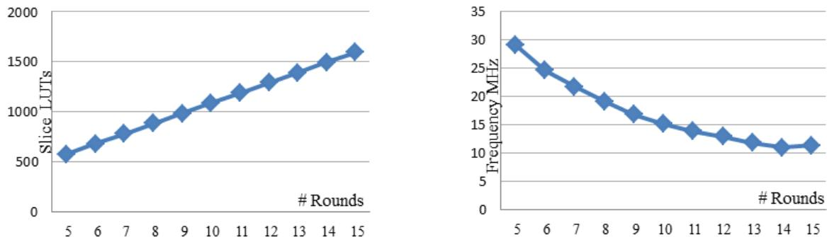
Fig. 2. FPGA implementation of the RC5 encryption algorithm with  $r$  rounds.
