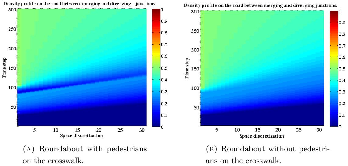
FIGURE 7. Traffic evolution on the main road between merging and diverging junctions of the roundabout.
