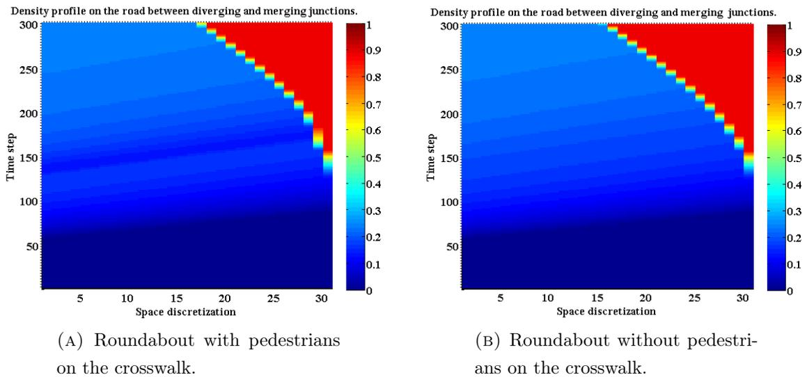
FIGURE 8. Traffic evolution on the main road between diverging and merging junctions of the roundabout.
