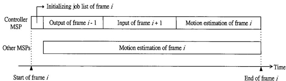
Fig. 7. Processing of a regular frame by MSPs.
