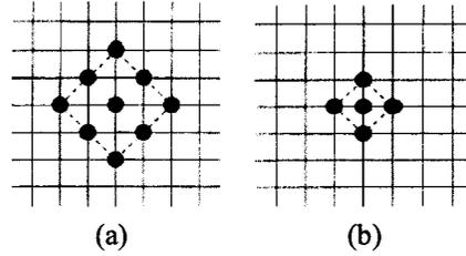
Fig. 3. Two search patterns of DS: (a) LDSP, (b) SDSP.
