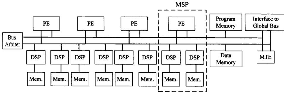
Fig. 2. Processor subsystem block diagram.
