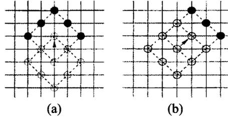
Fig. 4. (a) The LDSP moves upward; (b) the LDSP moves northeast.
