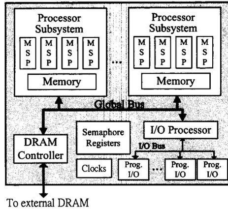
Fig. 1. MDSP block diagram.
