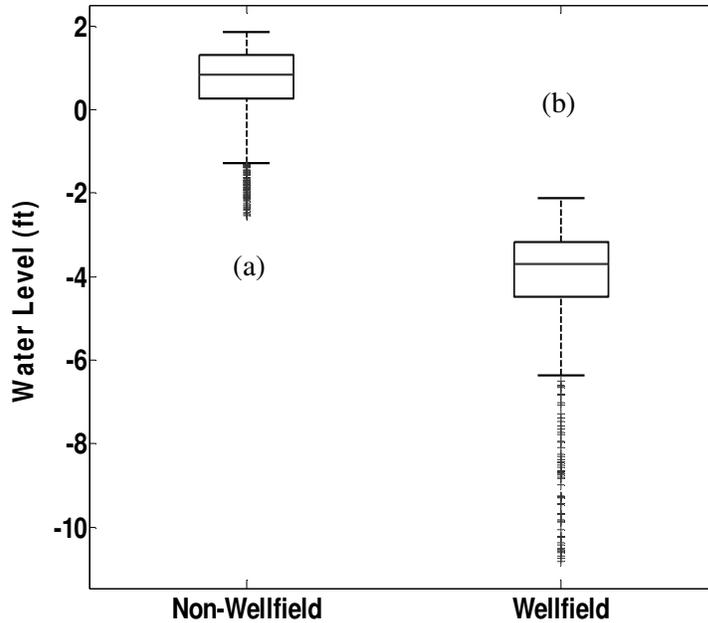
Figure 6. Water level fluctuation of two cypress wells; a) outside a well field and b) in a well field.
