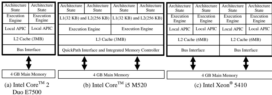
Figure 1: Target Intel multi-core processors.
