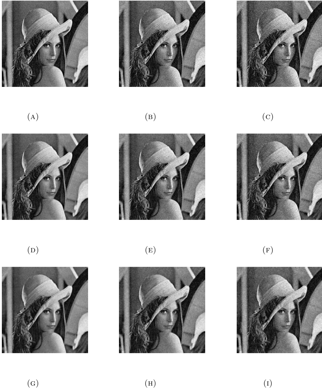
FIGURE 2. (top row) Noisy Lena images with different levels of Gaussian noise (A)-(C), \sigma^2 = 0.002, 0.004, 0.006 , respectively; (second row) (D)-(F) corresponding denoised images by model (2.3); (third row) (G)-(I) by model (2.4).
